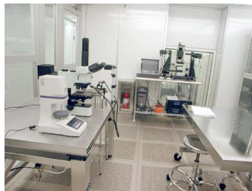
Fig. 3. Air-bearing table, direct thickness measure, bright field/dark field microscope, ellipsometer in ISO Class 4 lab.
